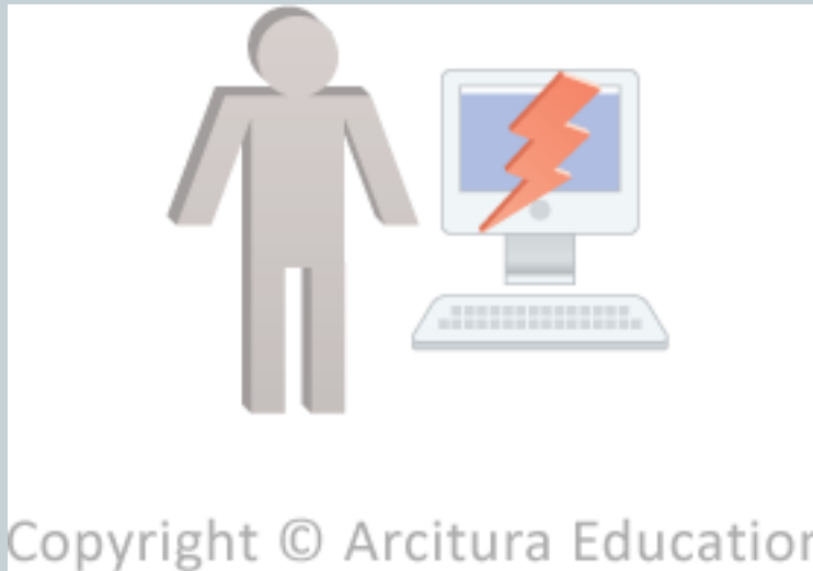
Figure 6.7 - The notation used for an attack originating from a workstation. The human symbol is optional.
